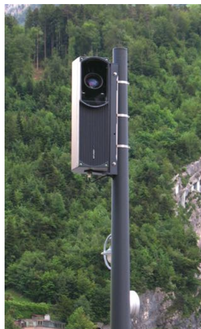
B Upright installation on pole with pipe clamps
